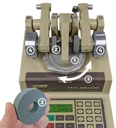
Material to be tested is placed on the rotating base.
